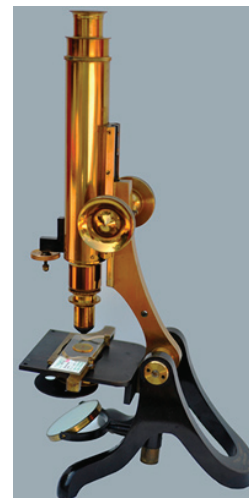
Fig. 1. An English, Henry Crouch microscope (c. 1880) similar to the type developed by J.J. Lister and used by J.B. Lister. This type was used from 1826 to the 1890s. Microscope picture from Alan Gillen's personal collection.
