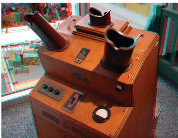
Fig. 2. An x-ray machine used to check shoe fit. The two views are one for the customer and one for a parent or spouse. Image courtesy of Wikimedia Commons, public domain, https://commons.wikimedia.org/wiki/File:Xray_for_shoes.jpg .
