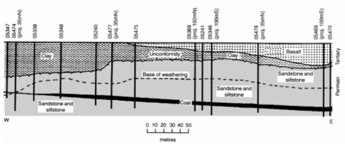
*Figure 3.* Simplified longitudinal, west-to-east cross-section through the Crinum Mine drift entries showing the geology and the exploratory drill-holes (adapted from the BHP Australia Coal Pty Ltd's Crinum Mine Project cross-section). The upcast ventilation shaft was excavated in the approximate position of Drill-hole 05469.
