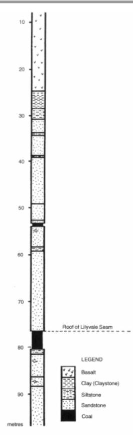
*Figure 4.* Geological log for Drill-hole 05469 showing the strata sequence intersected by the upcast ventilation shaft (adapted from the BHP Australia Coal Pty Ltd's Crinum Mine Project drill-hole log).
