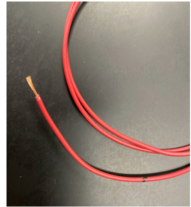
Figure 5: Mark and strip the wires on each end
