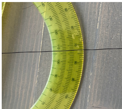
Figure 3: This reading indicates 73^\circ and 107^\circ , or an elevation of 17^\circ .
