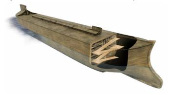
middle of the hull where bending stresses are highest. (This placement also better utilizes the irregular space at bow and stern.)
