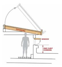
Any opening on the deck of a ship needs a wall (combing) to prevent water from flowing in, especially when the ship rolls. In this illustration, the window ends a cubit upward and above, as described in Genesis 6:16. The central position of the skylight is chosen to reflect the idea of a "noon light." This also means that
