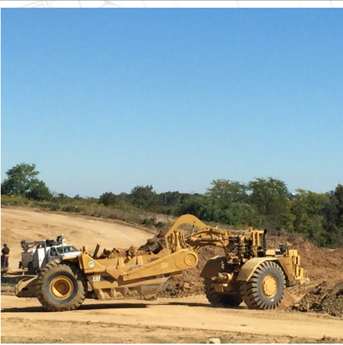
Large Caterpillar scrapers like this one can haul up to 50 yards of dirt at a time.
